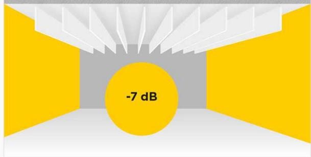
**Solution 2:** full cover with sound absorbing baffles
